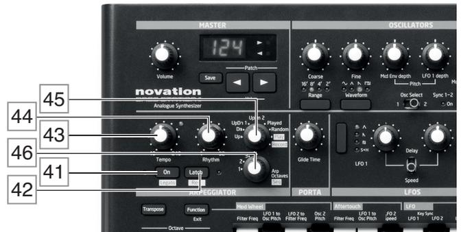
The Arpeggiator is enabled by pressing the **On** button **42**; the associated LED will confirm its status.
